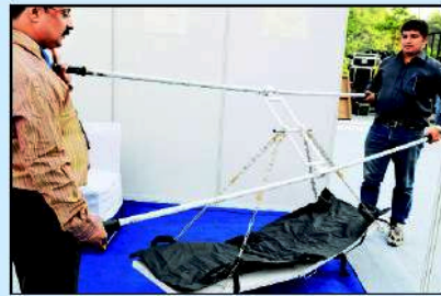
EASY STRETCHER: An add-on structure to make carrying the injured easier. All four corners can be moved independently while still keeping the stretcher in a horizontal position. Useful on stairs. Innovator | Mahesh Atale, MUMBAI
