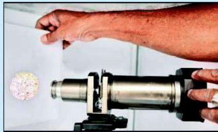
CHANDRA MICROSCOPIC SLIDE PROJECTOR: Specimen under microscope can be viewed by many at one time with this device. It is ideal for classroom learning where students otherwise have to wait for their turn Innovator | Chandra Narayan Bairagya, WEST BENGAL
